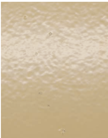
Pinholes are difficult to see under white light inspection.
